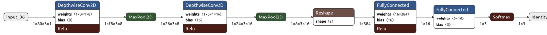
Figure 6.6: Model architecture for Depthwise-Separable Convolutional Neural Network with two DS-CNN layers of varying size.
