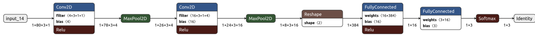
Figure 6.5: Model architecture for Convolutional Neural Network with two convolutional layers of varying number of channels.
